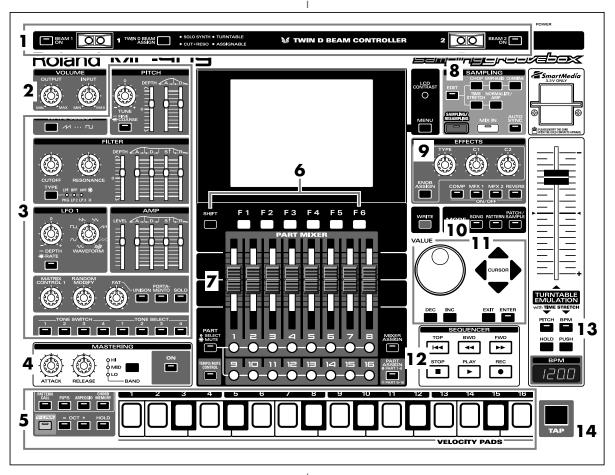
In the Sampling section of the panel, press [SAMPLING/ RESAMPLING] so the indicator is lighted. The Sampling Menu screen will appear.
